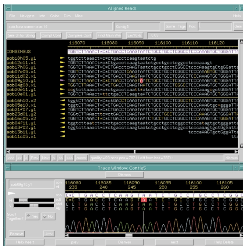
Figure 4 | Shotgun-sequence assembly. A key component of shotgun sequencing involves the computational assembly of redundant collections of sequence reads, from which an accurate consensus sequence can be deduced. Shown here is a representative display from the program Consed 18 , which is the viewing tool typically used with the associated base-calling program Phred 16,17 and sequence-assembly program Phrap. In this ~60-bp view from a shotgun-sequencing project, the indicated sequence reads have been assembled and used to deduce the consensus sequence (highlighted in white along the top). The primary data for one of the sequence reads (the sequence trace) is shown along the bottom. See REF. 18 for additional details about the various features of Consed shown here.
