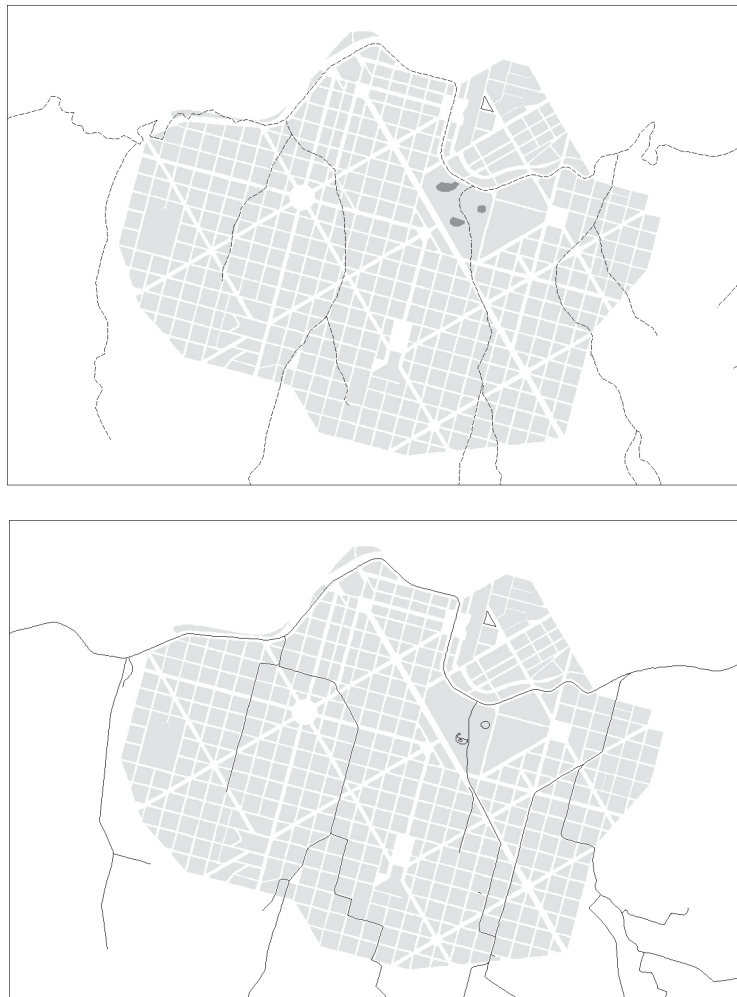
FIGURE 1. Plan of Belo Horizonte downtown, indicating the original (top) and current (bottom) stream courses.
